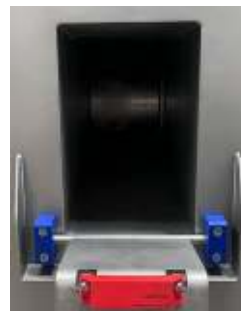
Hygienic zone shown in running position (closed) and in cleaning/inspection position. When opened, the grinder cannot be started until the guard has been positioned in closed position.
